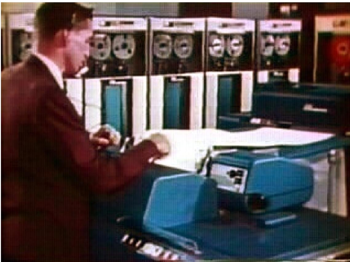
*Merge sort type algorithms allowed large data sets to be sorted on early computers that had small random access memories by modern standards. Records were stored on magnetic tape and processed on banks of magnetic tape drives, such as these IBM 729s.*
